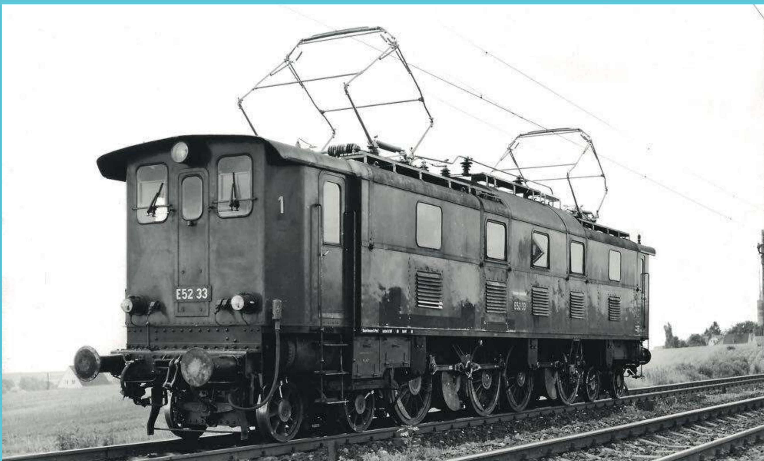
Elektro-Lok E 52 für den schweren Personenverkehr. The class E 52 electric locos were designed for heavy passenger traffic.
